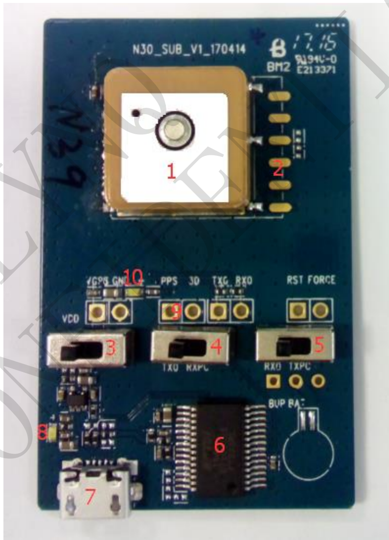
Figure 1-1 N30/N39 EVB Top View
